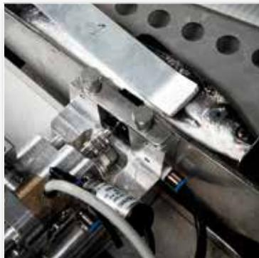
Fish in position for vaccination. A camera system controls the vaccination units, adjusting injection point and depth to every single fish. The accuracy is above 98%.
