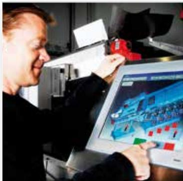
Only one operator is necessary to operate the machine, which is controlled by an operator panel. The machine also communicates with the operator via voice messages.
